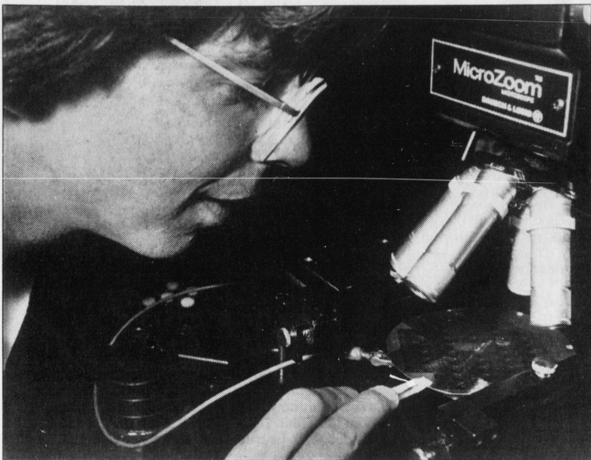
Prof. James Burr carefully positions a silicon wafer containing low-power test circuits. The circuits use a thousand times less power than conventional circuits to accomplish basic tasks like addition and memory storage. Burr hopes these simple devices will eventually lead to much smaller and faster computers.
